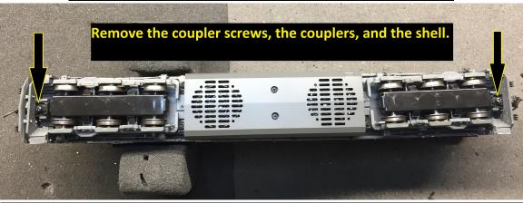
Hold the model by the fuel tank over something soft, and press down on the steps, alternating end-to-end until the shell comes free.
