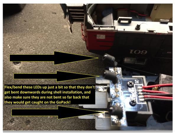
Hold the shell upside down in one hand, and insert the chassis with the other (headlight/ditch lights first). Insert the couplers and screws, and then test the model on the layout.
